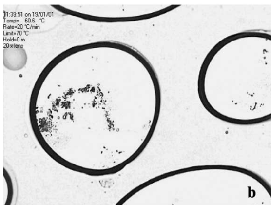
Fig. 3. HSM pictures of felodipine crystals after melting of the excipients: cetanol (a) and cetanol + Pluronic® F127 (b) particles.
